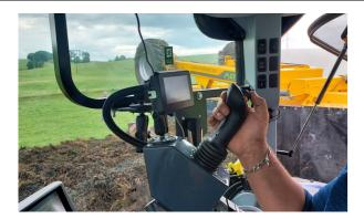
All movements are controlled from inside the cab using a touch screen and joystick.
