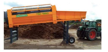
TSC screens are compact, all-in-one screening machines. Their simple, efficient design provides all the essential functions for quality screening. Maintenance operations are minimal.
